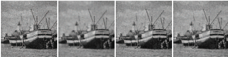
Figure 11: (Left to Right) Noisy image of the Boats perturbed by Gaussian additive noise of zero mean and variance \nu = 0.01 . Filtered image of the Boats after 17 iterations by the finite difference method. Filtered image of the Boats after 5 iterations by the finite element method. Filtered image of the Boats after 7 iterations by the mimetic discretization method.
