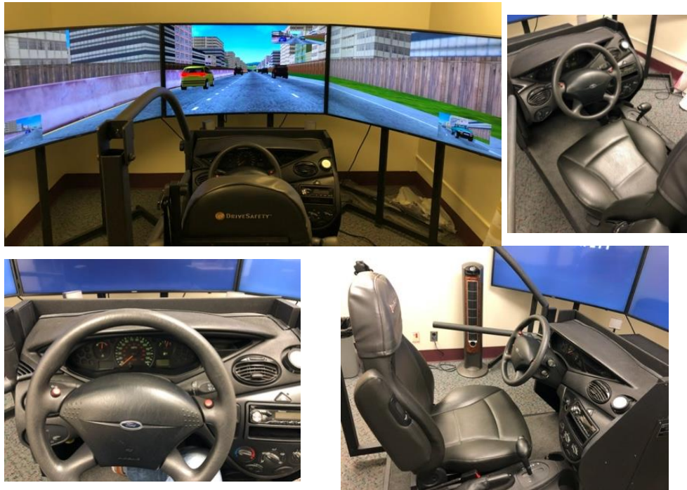
Figure 1. SDSU Smart Transportation Analytics Research (SDSU-STAR) Lab driving simulator
