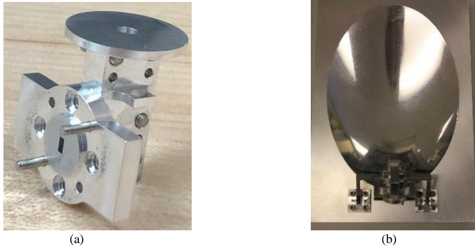
Fig. 8.1. Photograph of the fabricated (a) proposed feed horn antenna and (b) the offset parabolic reflector with feed horn assembly.
