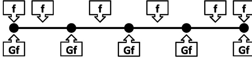
Figure 4: CGM Gradient,  $f$  denotes the locations that the data must be held and  $Gf$  shows the location where the gradient is calculated using CGM Gradient operator.
