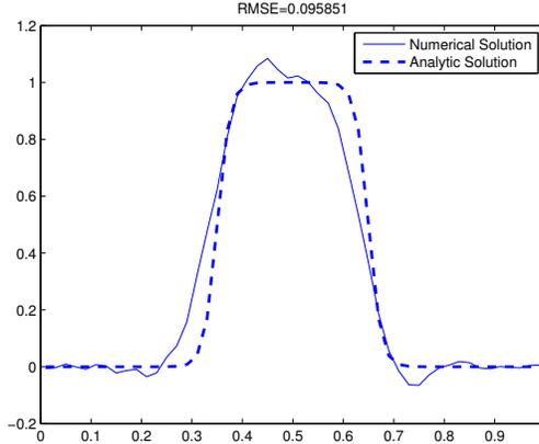
Figure 3: Second Order Accurate CGM Divergence Operator with Sixth Order Interpolation Scheme,  $Cr = 1.1$ .
