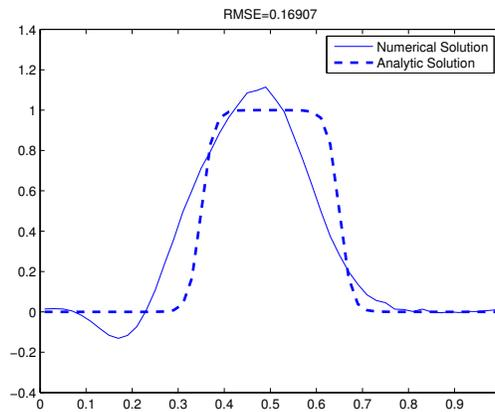
Figure 7: Second Order Accurate CGM Gradient Operator with fourth Order Interpolation Scheme using V1 approach,  $Cr = 1.65$ .
