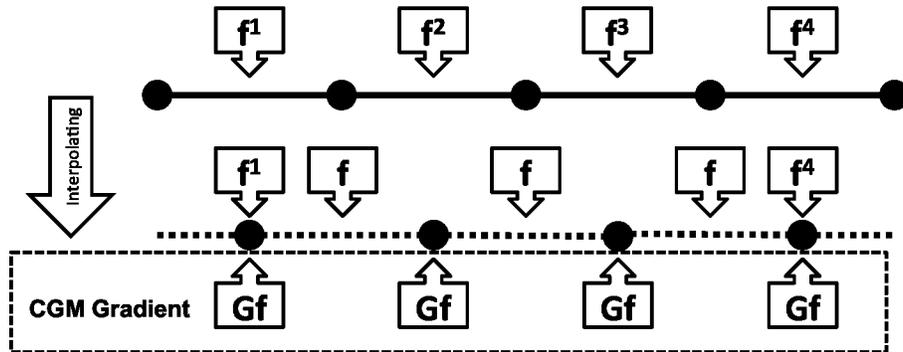
Figure 6: V2 Approach: Data is interpolated to all the interior nodes. CGM gradient operator is used to calculate the gradient at the cell centers directly. Hence, there is no need to interpolate the calculated gradient.
