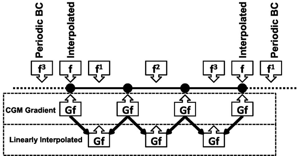
Figure 5: V1 Approach: Data is located at the cell centers only. Using the boundary condition data is interpolated at the boundary nodes to satisfy the grid requirements of the CGM gradient operator. The gradient is calculated then at the nodes and linearly interpolated to the cell centers.
