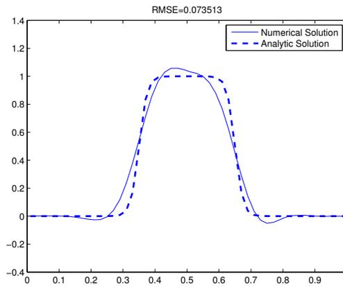
Figure 9: Second Order Accurate CGM Gradient Operator with fourth Order Interpolation Scheme using V3 approach,  $Cr = 1.2$ .
