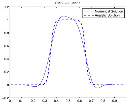
Figure 2: Second Order Accurate CGM Divergence Operator with Forth Order Interpolation Scheme,  $Cr = 1.2$ .
