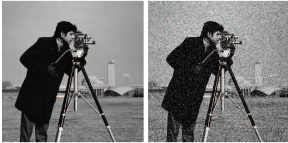
Figure 3.12: (left to right) Noise-free image of the Cameraman along with the noisy image of the Cameraman which has been perturbed by Gaussian white noise with zero mean and variance 0.01. The correlation coefficient between the noise-free image and the noisy image, \text{corr}(f, u_0) , is 0.9280.
