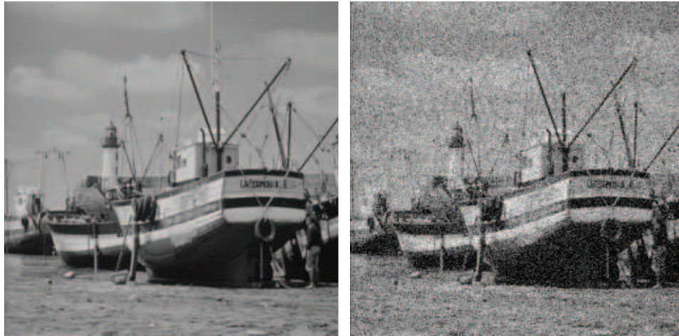
Figure 3.8: (left to right) Noise-free image of the Boats along with the noisy image of the Boats which has been perturbed by Gaussian white noise with zero mean and variance 0.01. The correlation coefficient between the noise-free image and the noisy image, \text{corr}(f, u_0) , is 0.8692.
