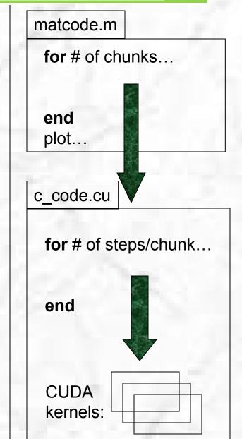
Vectors transferred to GPU, then do chunk of time steps:
