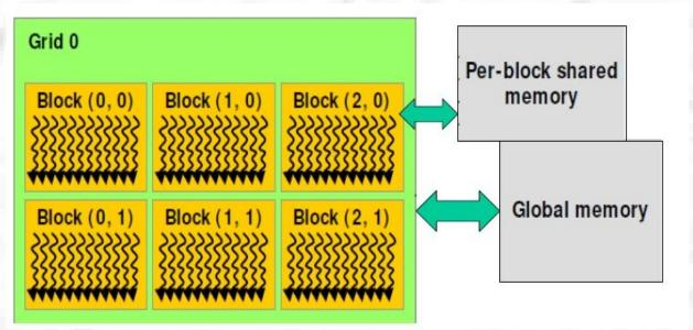
Threads instantiated through calls to a "kernel" Thread synchronization within blocks Each thread typically computes one cell of array or matrix Each thread has access to per-thread local, per-block shared, and global variables.
