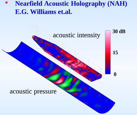
Reconstruction of the acoustic field in the surface of the structure from surface pressure measurements.
