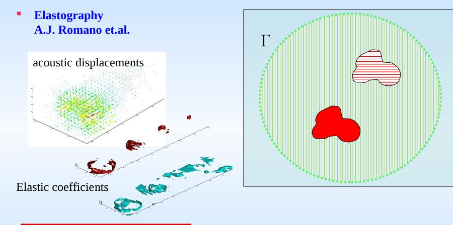
Reconstruction of elastic properties inside the structure from volumetric displacement measurements.
