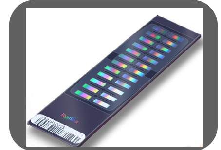
2005 - 100K Beadchip 2008 – duo 1M BeadChip 1M tests/ slide 1M answers/hour
