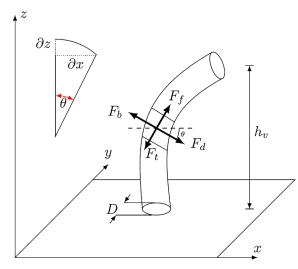
Physics forces accounted for on a single vegetation branch.  $F_b$  is the buoyant force,  $F_f$  is friction,  $F_d$  is drag, and  $F_t$  is tension.  $h_v$  is effective height, D is the diameter, and  $\theta$  is the angle of deflection.
