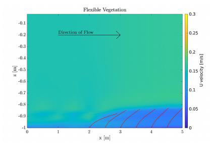
Comparison of rigid versus flexible vegetation and the flow fields generated around them. The flow in these images is 0.2 m/s left to right. The rigid field acts as a step, pushing water up and around the field, while the flexible vegetation absorbs some of the momentum and bends to smooth the passage of the fluid.
